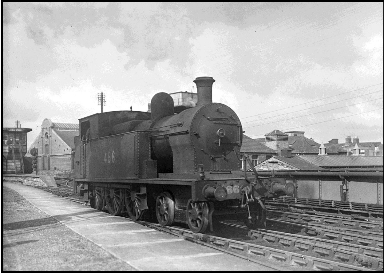
Ex-CB & SC B4 class 4-6-0T No. CIE 466 at Dublin, Amiens St c1950s (65092)
